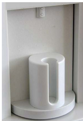
Figure 6. Sample tube adapter—supporting BD Vacutainers and Sarsted Monovette (3.5ml)
