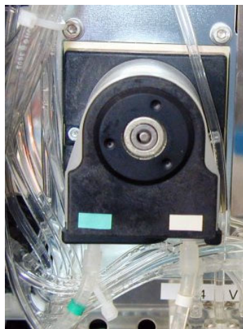
Figure 12. Peristaltic pump after replacement of tube
