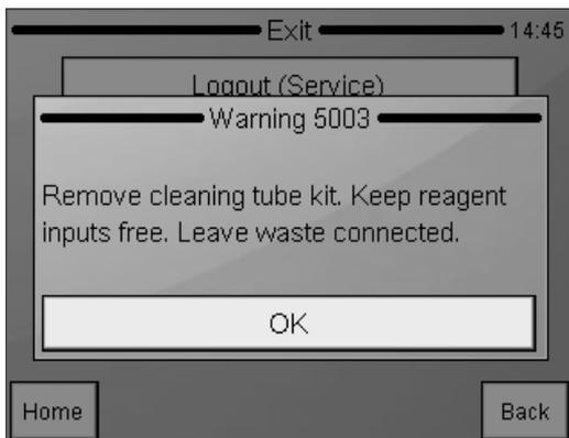
As a next step, the analyzer asks you to remove the cleaning tube kit. Leave Waste connected.
