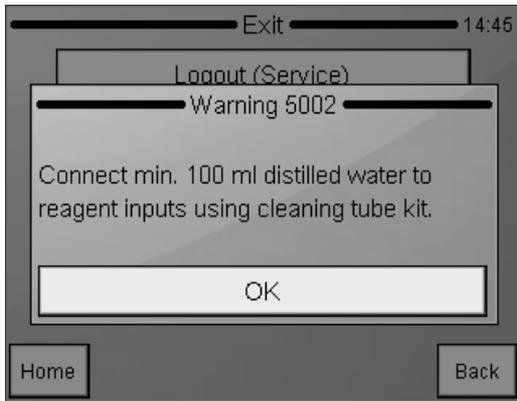
Next, you should connect the cleaning tube kit to the reagent inputs, submerging the free end in a bottle containing at least 100 ml of distilled water.
